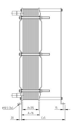
PLATE HEAT EXCHANGER GC-28P DIMENSIONS, MM
